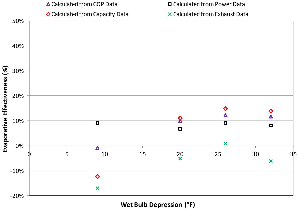
FIGURE 20. EVAPORATIVE EFFECTIVENESS CALCULATED WITH FOUR METHODS VS. WET BULB DEPRESSION FOR PRE-COOLER C
