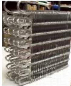
2. Serpentine tube dogbone fin HX: Low-cost, wide fin spacing (no enhancements), continuous tube (no leakage potential)
