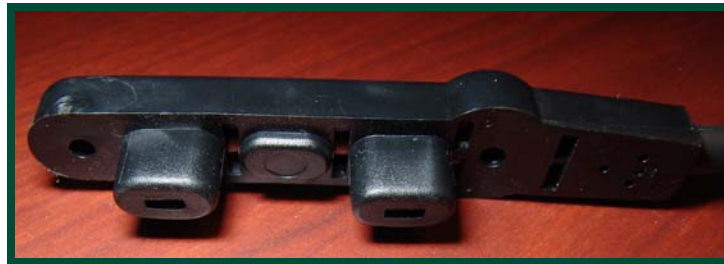
FIGURE 7. DOORFRAME MATING PLUG WHICH PROVIDES POWER TO DOOR HEATERS
