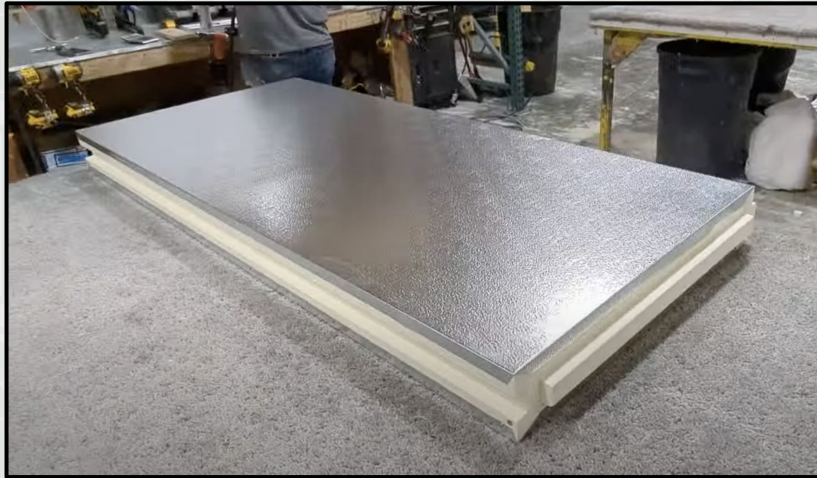
Vacuum Insulation Panel (R-Value > 90)
