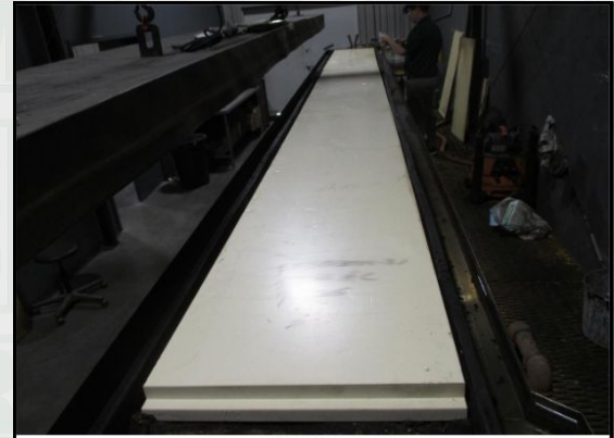
Photo No. 4 Post-Test Unexposed Side
