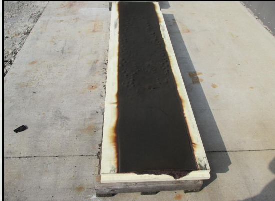
Photo No. 6 Post-Test Exposed Side (Middle Section)
