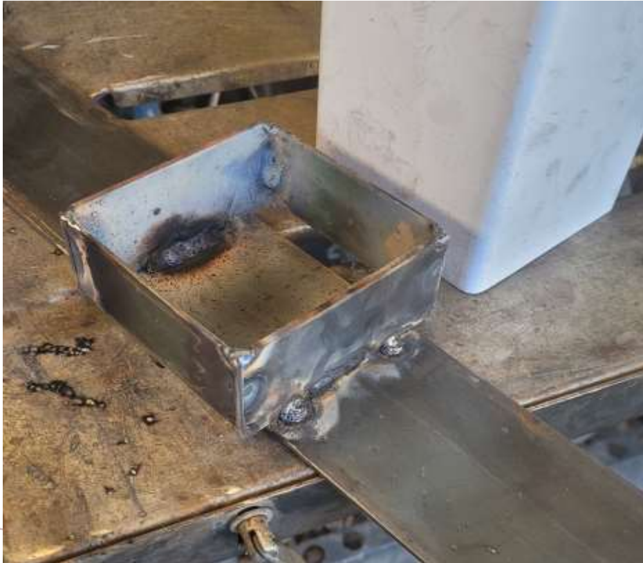
Supports for the Vinyl Fence
