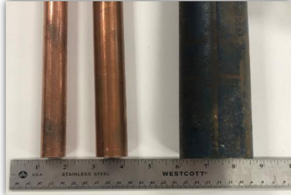
7/8" and 1-1/8" Copper vs 2" Steel
