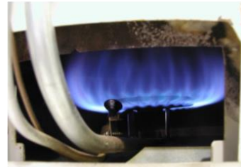
Ultra-Low NOx Water Heater Burner (< 10 ng NOx/J)
