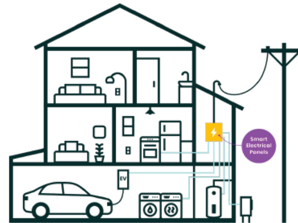
Smart Electrical Panels
