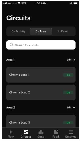
The contactor behind a breaker can be controlled by selecting the breaker and then toggling the selector in the upper righthand corner. If the breaker was assigned as "Always on" during installation the selector will be grayed out.
