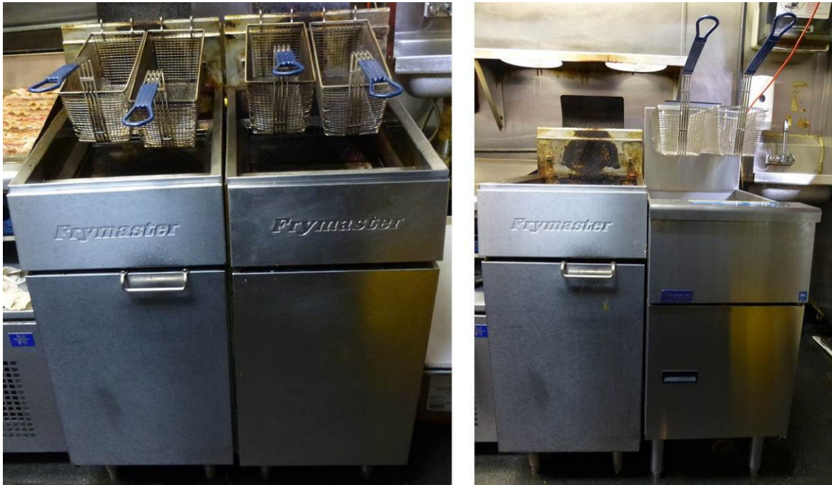
FIGURE 25. NORM'S PLACE FRYERS: PRE-EXISTING FRY BANK (LEFT PHOTO ) AND FRY BANK WITH REPLACEMENT FRYER (RIGHT PHOTO)
