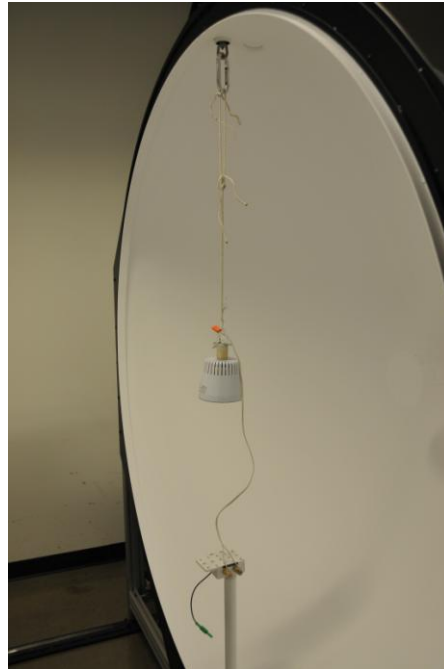
FIGURE 1. LUMINAIRE SETUP IN INTEGRATING SPHERE
