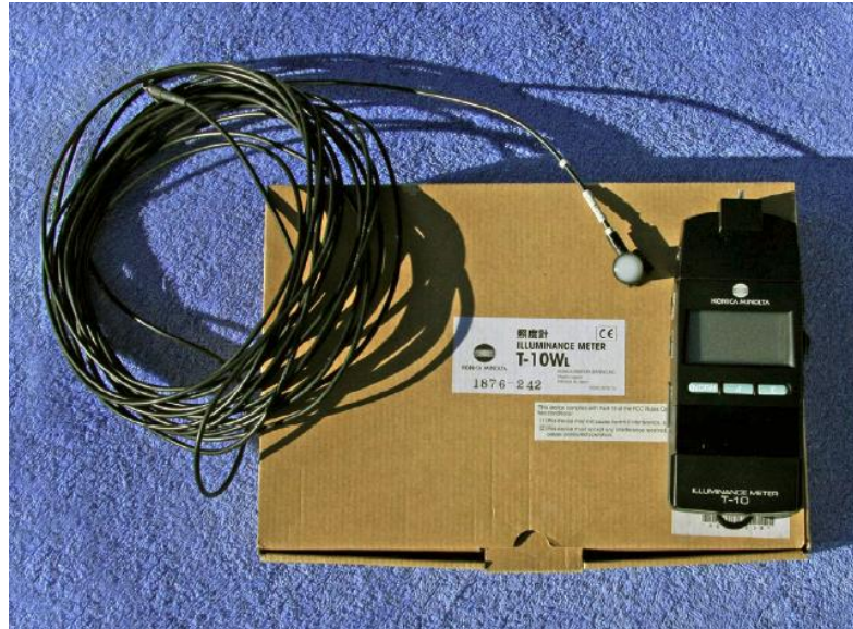
FIGURE 3. MINOLTA T10 LIGHT METER WITH WATERPROOF CABLE AND SENSOR
