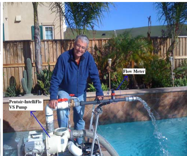
Figure 4: Hydraulic cleaner test setup
